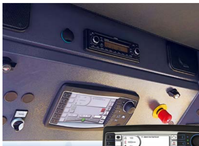
Operating and health status data: operating data are displayed for the driver on large and clearly structured displays.
