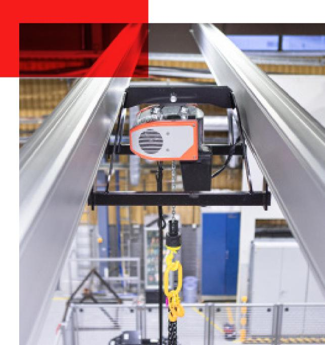
**Konecranes** C-series electric chain hoist C-series electric chain hoist **Konecranes** 3
