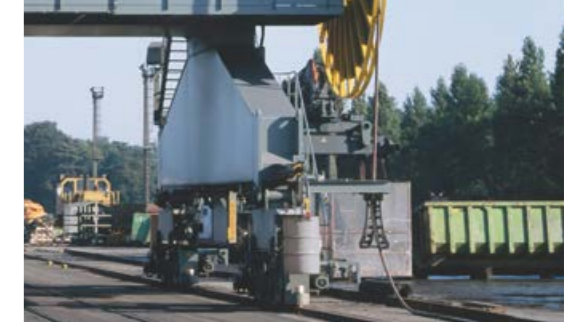
The cable guide section helps everything to run smoothly, even when the direction of travel changes.
