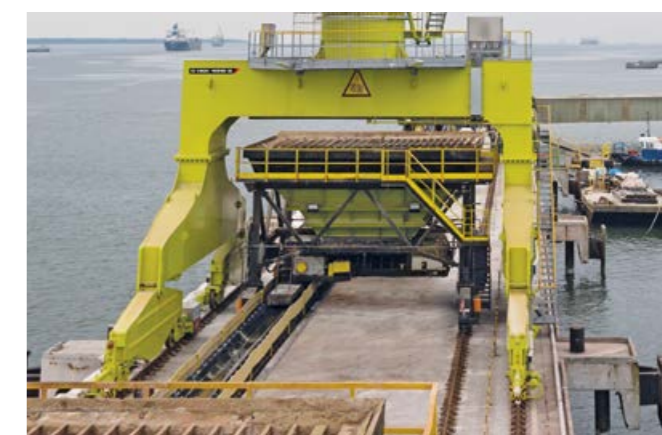
Efficient use of space permits excellent maneuverability of the hopper under the portal on narrow and quays off the shore.
